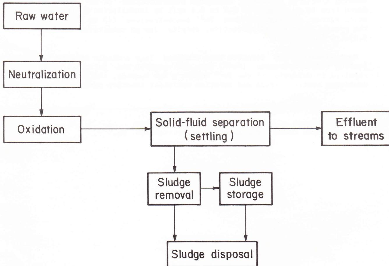
FIGURE 1. - Standard AMD treatment process.
