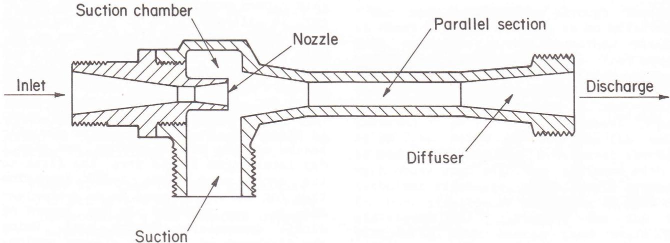
FIGURE 3. - Jet pump diagram.
