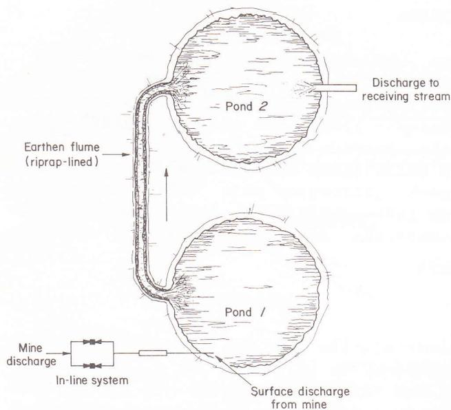
FIGURE 5. - Schematic of test site.
