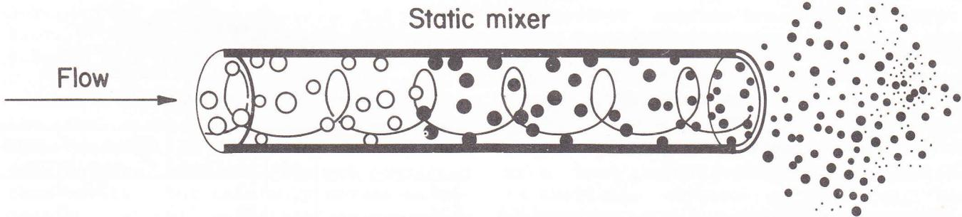
FIGURE 4. - Static mixer diagram.
